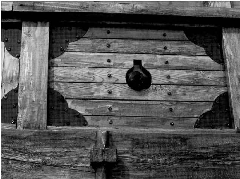
The gunports on the turtle ship at Noryang. Note also the simple iron reinforcements, which may have given rise to the claims that the turtle ship was an ironclad battleship.
